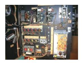
The ship unit was dirty and had some broken contacts which explains why no ships were getting hit. I soldered new contacts to the old assemblies as
